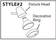
Style#2 - Install proper bulb type and wattage. Install decorative ring.
