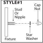
STYLE#1- Tuck electrical wires into outlet box and position fixture over studs or nipple on mounting bracket assembly. Secure fixture in place with star washer(s) and cap nut(s). Note: If required, assemble body and
